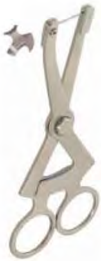
SS-1444 Clamp, Osteometer Length about 155 mm, ridge width measurement, two-sided scale, measuring range 0 - 25 mm
